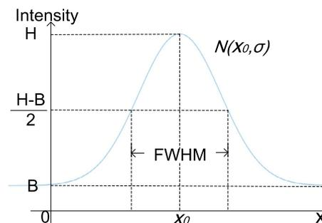
Fig. 6 FWHM of normal distribution  $N(x_0, \sigma)$  of star profile.  $B$ ,  $x_0$ , and  $H$  indicate the average intensity of the background, the center position of the star, and the intensity of the star center, respectively
