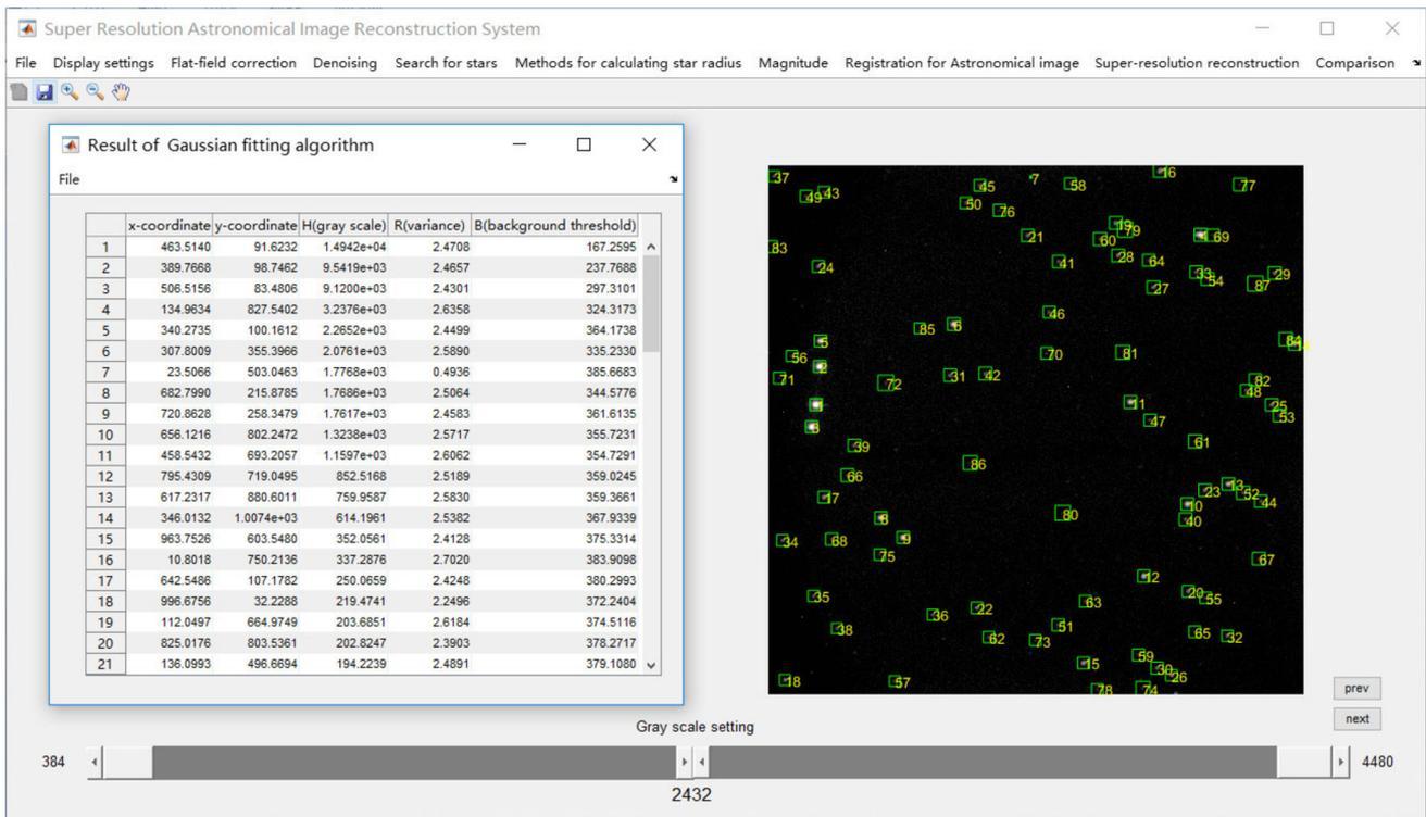
**Fig. 7** Automatic star searching and centering for reference image. The searched stars are marked by green squares and numbered in yellow in the right sub-window with their position parameters listed in the left window
