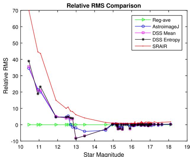
**Fig. 15** Relationship between relative RMS contrast and star magnitude. To better show the differences, the relative RMS contrast is used, which means the RMS from the Reg-ave is subtracted to all corresponding RMS contrast values
