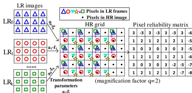
Fig. 4 HR grid and definition of pixel reliability
