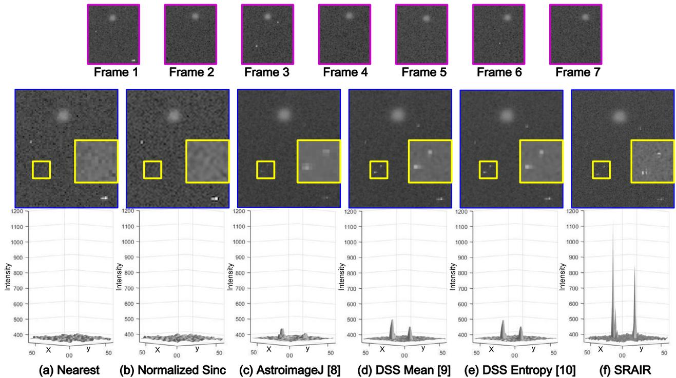
**Fig. 11** Comparison of output images from different techniques. Top row: Seven input frames, where Frame 1 is the reference frame. Middle row: Twofold-magnified results of different methods. The local areas, which contain two white points from Frames 3 and 6, are magnified
